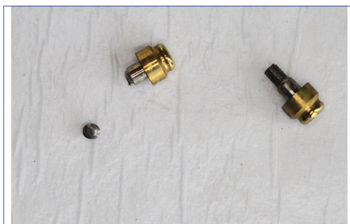
[Table/Fig-3]: Images of the fractured and loosened abutments.
